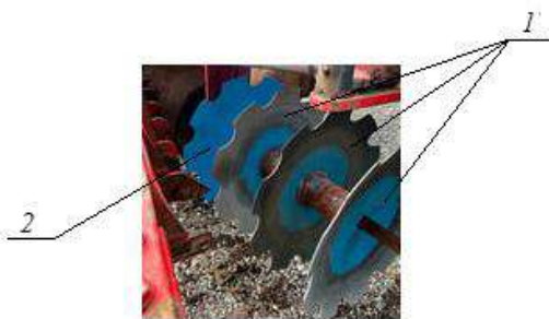
Figure 2. Installed testing discs on the harrow before field testing: 1) three coated discs; 2) uncoated discs.
