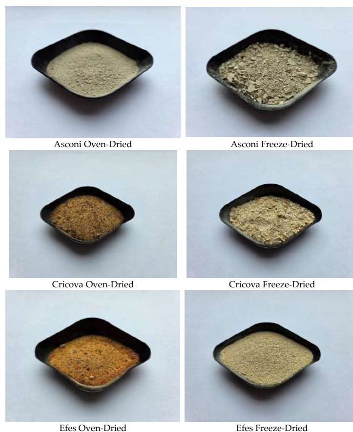
Figure 3. Digital images of lees and spent brewer's yeast samples dried by the two methods.
