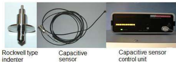
Figure 4. Main elements of the CETR UMT-2 tribometer for microindentation testing
