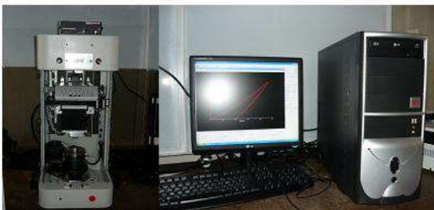
Figure 2. The CETR UMT-2 tribometer for standard scratch and microhardness testing, connected to a computer.
