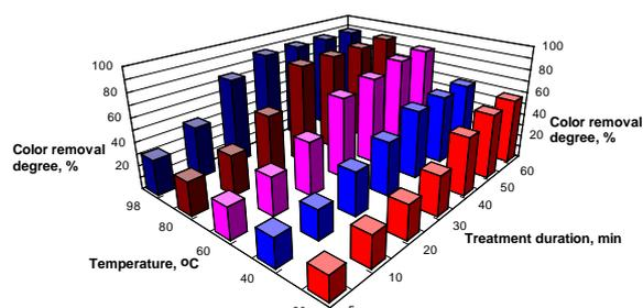
Figure 6. Discoloration degree for Acid Red 6
