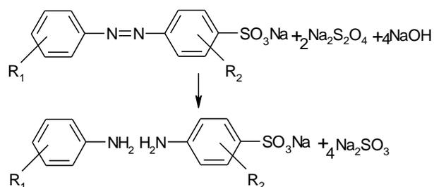
There are opinions that the dithionite ion may be understood as two sulfoxyl ( $\text{SO}_2\cdot^-$ ) radicals joined by a 2.39 sulphur-sulphur bond, that is significantly longer (and hence weaker) than a typical S-S bonds; thus,  $\text{S}_2\text{O}_4^{2-}$  will easily dissociate into two free radicals  $\text{SO}_2\cdot^-$ :
